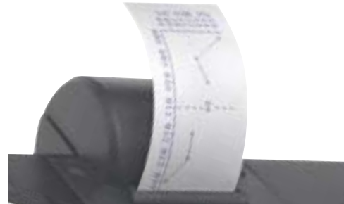
There's an integral 16-column printer for hard copy data. A feature of the LaserCM is the on-board printout data graphing option developed to support predictive maintenance procedures.
